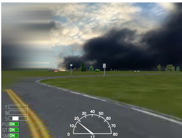
Figure 5 Void filling using linear interpolation between adjacent color and average color on pixel-line basis.
