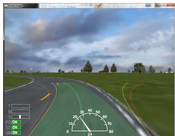
Figure 6 Illustration of the overlay for the predictive display.
