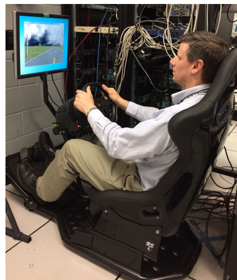
Figure 10 Operator station consisting of a seat, display and controller.
